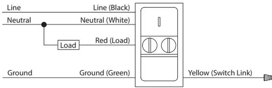
WLS 1 (Master / Master) Three-way Wiring - up to maximum 4 sensors can be grouped via "Switch Link"
