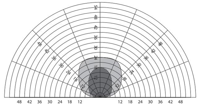
— Ultrasonic Tangential and Radial Coverage
